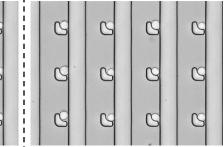
Wash uncaptured cells and add 70 µL of the medium into ! Inlet Well to prevent backflow. The #1.5 coverslip glass bottom (~0.17 thickness) mm compatible with DIC, TIRF, FRET, confocal microscopy, and widefield fluorescence.
